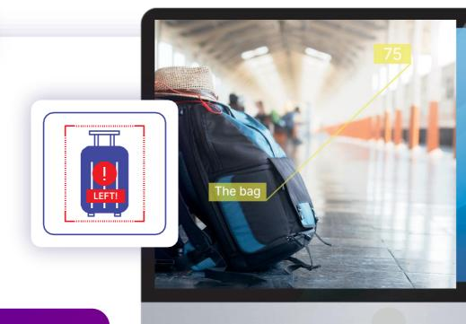
Works on the basis of unique object characteristics. After performing basic heuristics over the tracks, it determines the object's owner (using motion patterns and proximity to the object), whether the owner has stepped out of the frame or has moved away a certain distance
